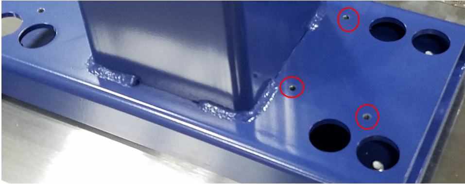
Figure 7. (6) holes in metal base line up with plastic
