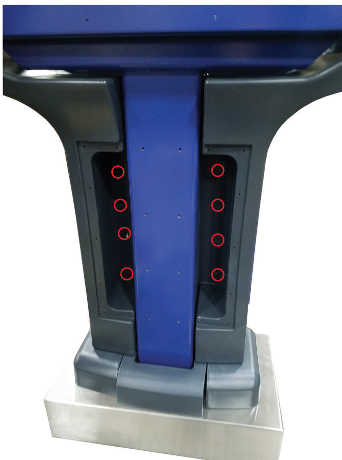
Figure 14. Back of the Auto Sentry® Petro, tighten 8 screws
